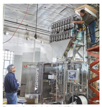
The combination weigher feeding into this XYRJ bagger presents an end user with thousands of potential combinations for accuracy within a fraction of an ounce. Watch this video to see the bagger in action: www.pwgo.to/3189.
