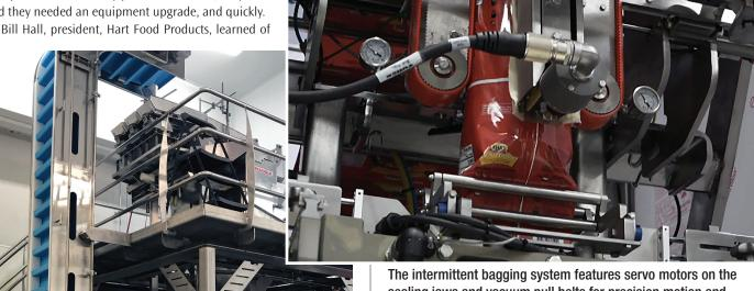
sealing jaws and vacuum pull belts for precision motion and performance. Rejects are down from 5% to less than 0.1% with the precision weigher and bagging system.
